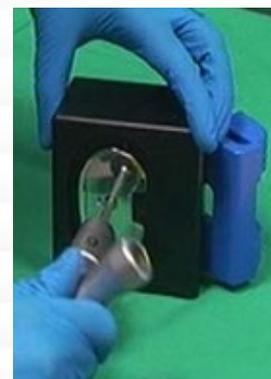
With the tibial implant in place, rotate the mounting bracket again by 90°. rotate and place the bushing between the implant surface and the table. place it. Mount the stem by rotating it by hand on the offset Please check (C). On offset using 12Nm wrench Tighten the stem. (D).
