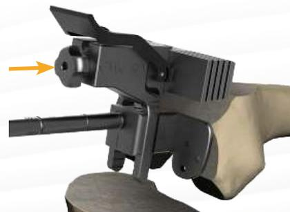
Setting piece movement distance from distance from +2mm to -10mm (orange rectangle).
