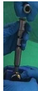
Combining 6Nm torque wrench and extension on offset Tighten the stem.
