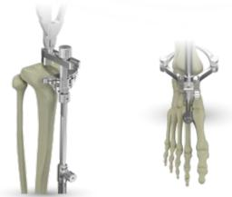
In the sagittal plane, the tibia mounting axis is both proximal using the slide settings at both distal ends with the mounting axis parallel to the anterior tibial shaft Then tighten the screw for both adjustments.
